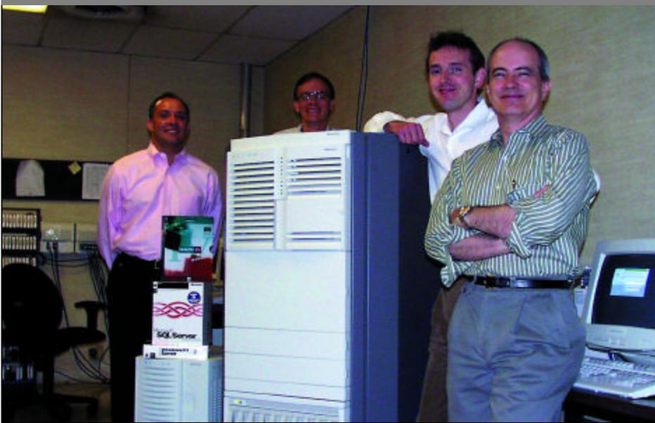
In preparation for the implementation of ERP, members of the IS department installed a new Data General Aviiion file server with three Intel Pentium Pro 200 processors and a 61 GB Clariion disk array. The smaller fail-over server is a Data General Aviiion with dual Intel Pentium Pro 200 processors. Pictured from left: Chuck Sharp, director of IS, Orin Owen, Iain Jarvis, and Keith Wallace.
